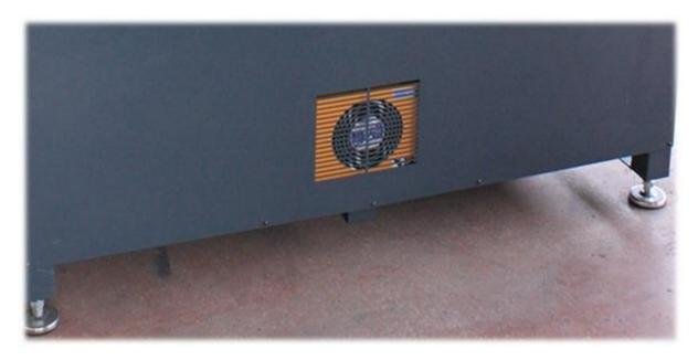
With the oil cooling unit in our presses, the machine automatically cools the hydraulic oil when the temperature exceeds the one you specify, and thus you will not experience any power loss and your felt life will be extended.
