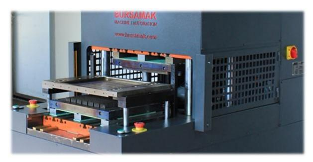
Hydraulically operated center and side ejectors allow you to automatically eject products from the mold. This significantly reduces production time and increases production volume.
