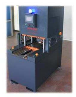
All hydraulic and electrical components of our presses are self-contained, allowing them to take up minimal space in your production area.
